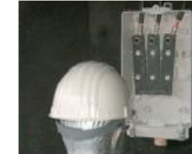
HELMET TEST before arc flash incident
