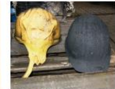
FOR COMPARISON: thermoplastic electrician's helmet and BOP Energy 3000 after the arc flash incident
