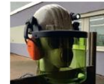
ARCSHIELD before arc flash incident
